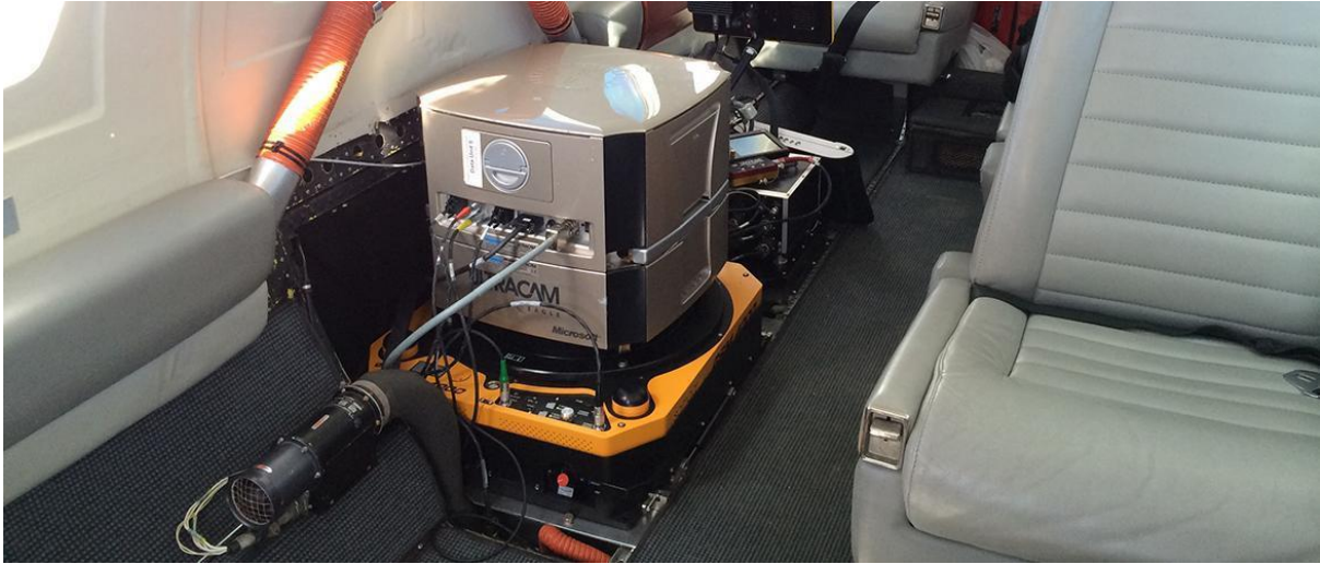
Figure 1 Photo of a survey-grade aerial camera with IMU in action
