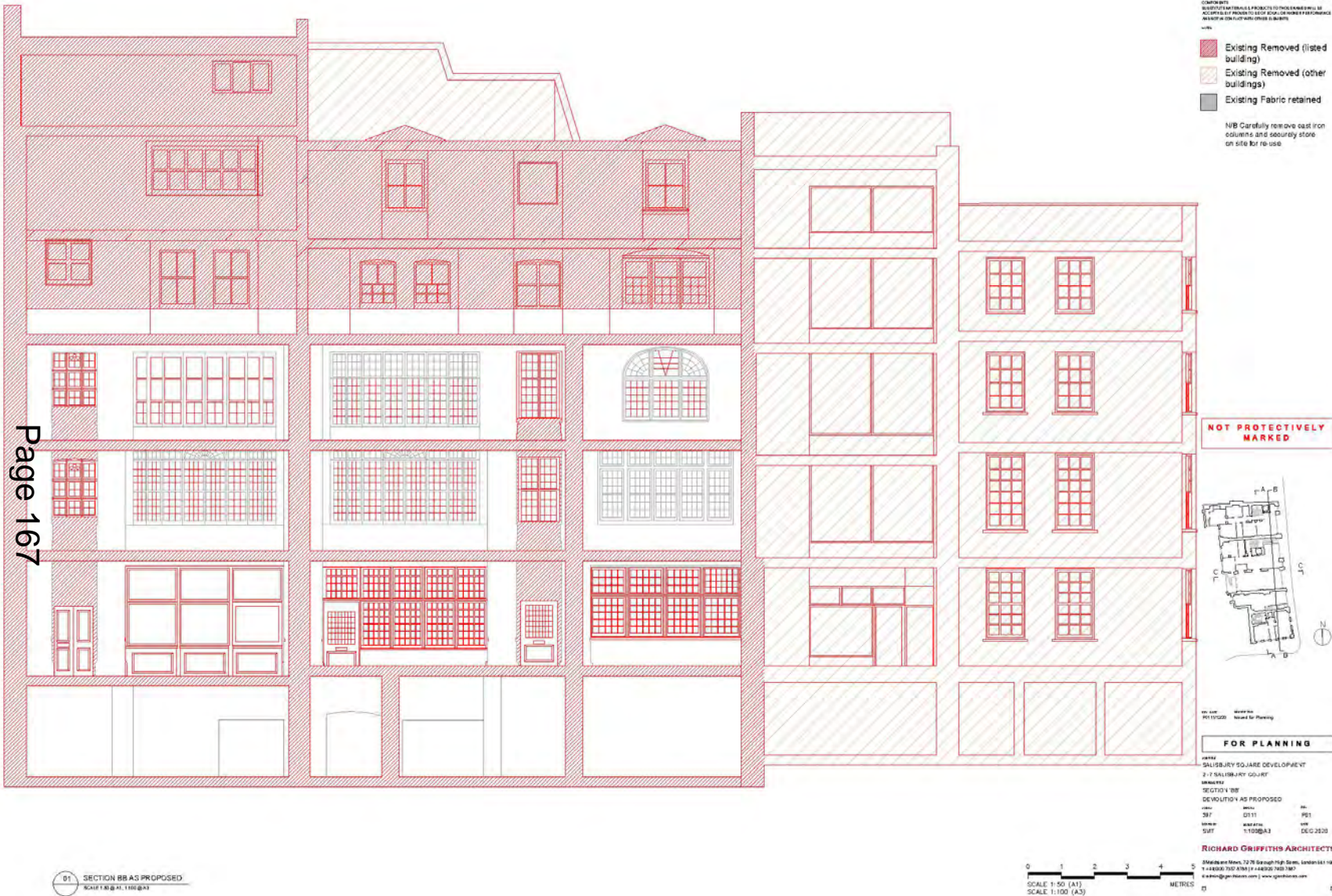
Proposed demolition section
