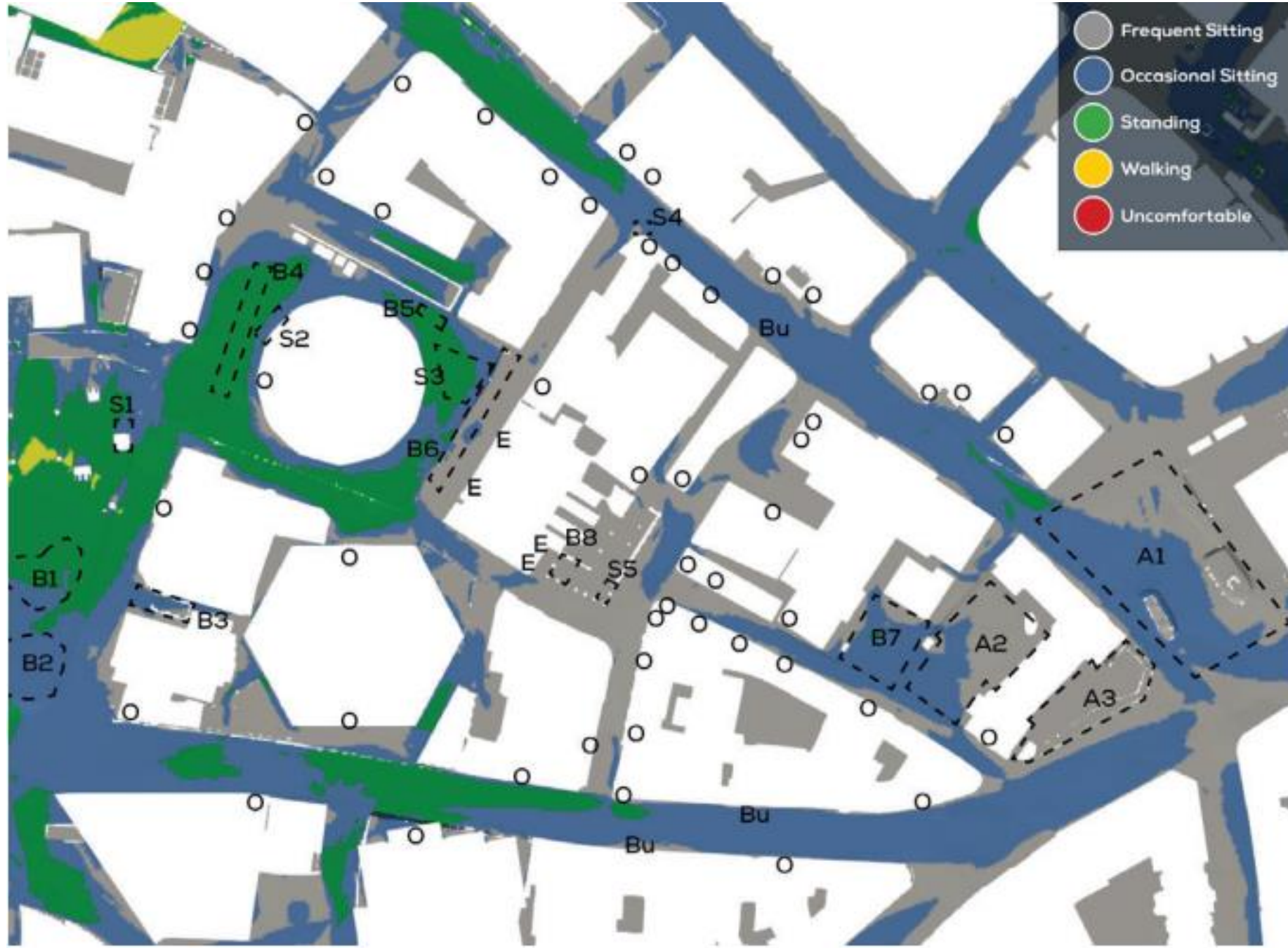
Windiest Season Conditions at Ground Level, Configuration 5 (Proposed Development with Tier 1 & Tier 2 Cumulative Surrounds)
