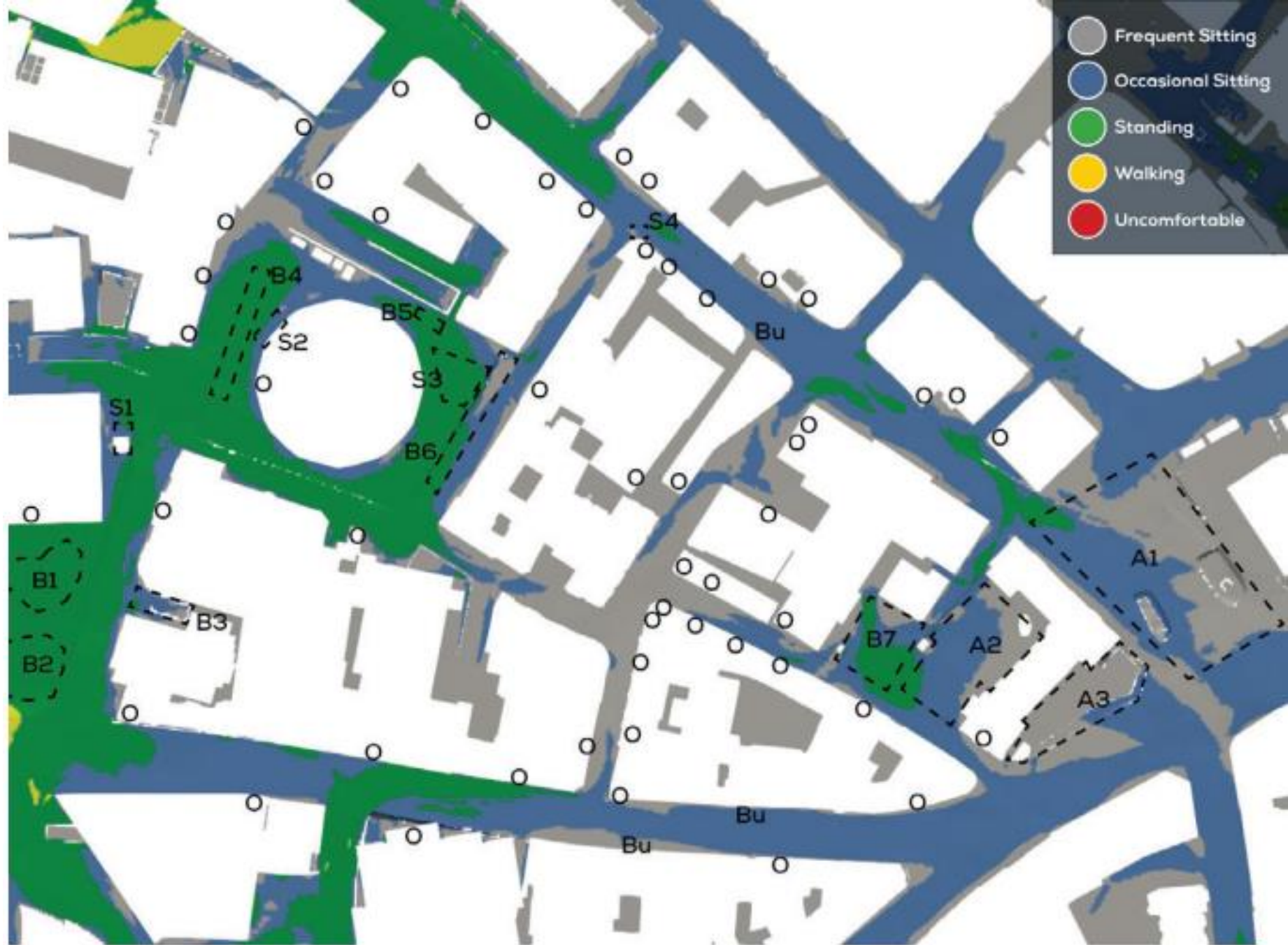
Windiest Season Conditions at Ground Level, Configuration 1 (Existing Building with Existing Surrounds)
