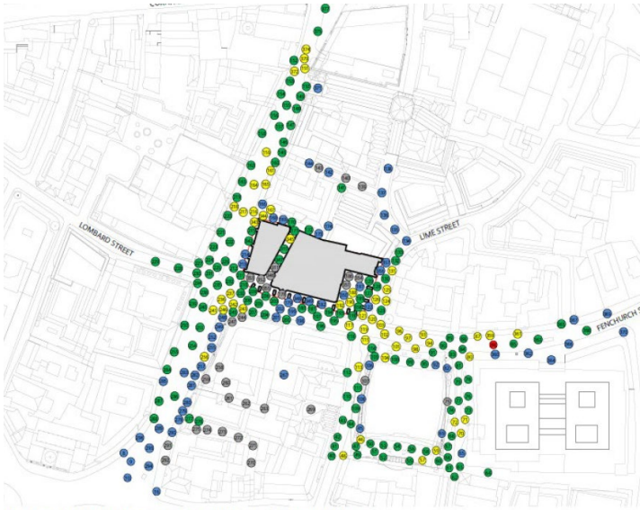
Pedestrian Wind Comfort Conditions - Ground Floor Configuration 6: Proposed Development with Existing Surrounding Buildings, Proposed Landscaping and Wind Mitigation Measures Windiest Season
