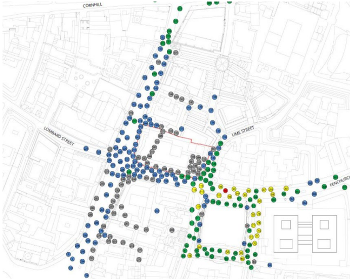
Pedestrian Wind Comfort Conditions - Ground Floor Configuration 1: Existing Site with Existing Surrounding Buildings Windiest Season
