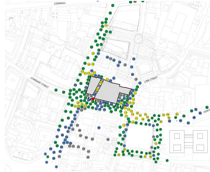
Pedestrian Wind Comfort Conditions - Ground Floor Configuration 7: Proposed Development with Consented Cumulative Schemes, Proposed Landscaping and Wind Mitigation Measures Windiest Season
