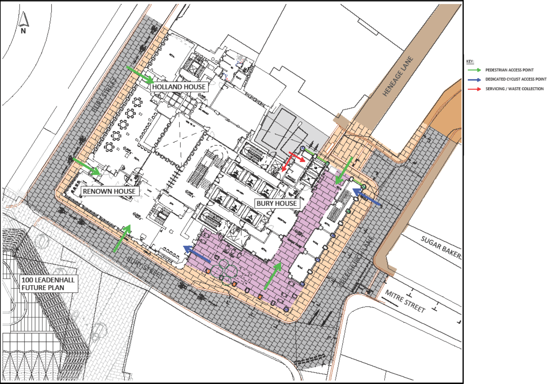
Proposed Servicing arrangements and cycle access
