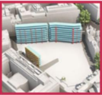
Partial retention of structure and facade
