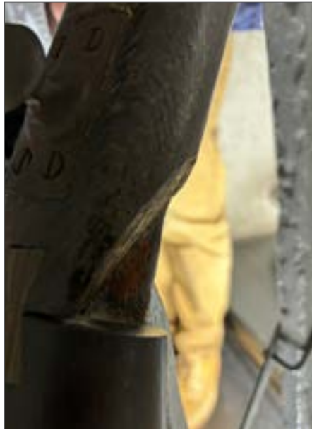
Fig. 45 Damaged section of handrail, 2024
