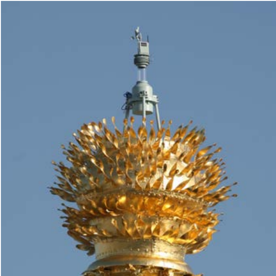
Fig. 79 Redundant panoramic camera & weather station installation at the top of the flaming orb, 2009
