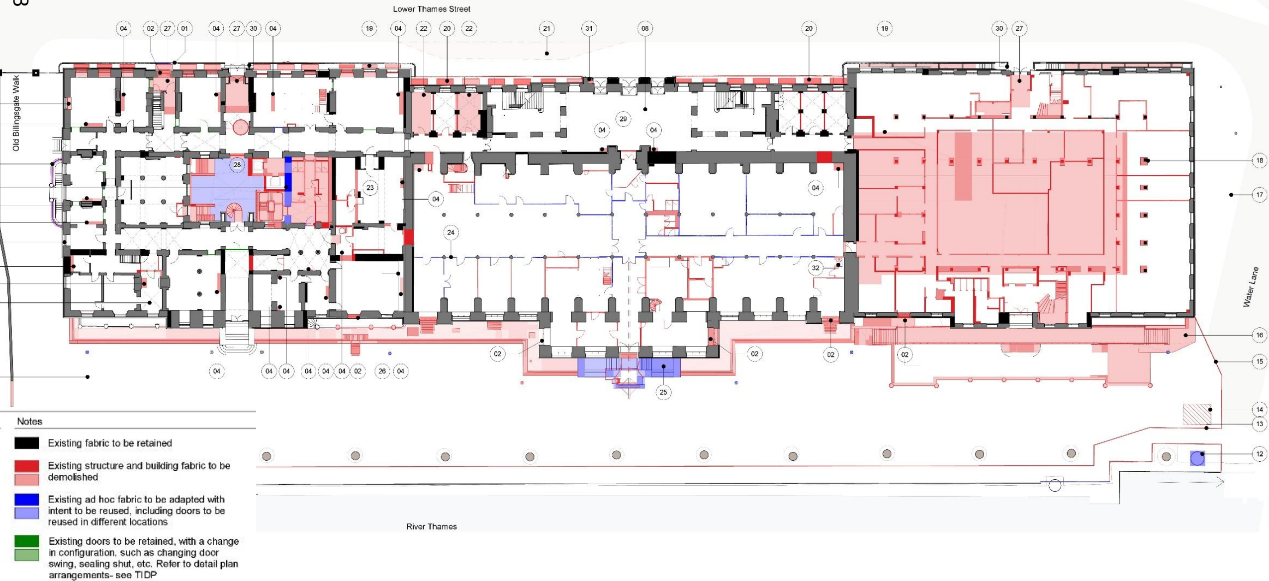
Demolition Ground Floor Plan
