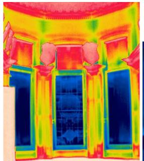
Figures 44 & 45. IRT images showing heat loss via the single glazed windows in the Stock Room and the Court Room.
