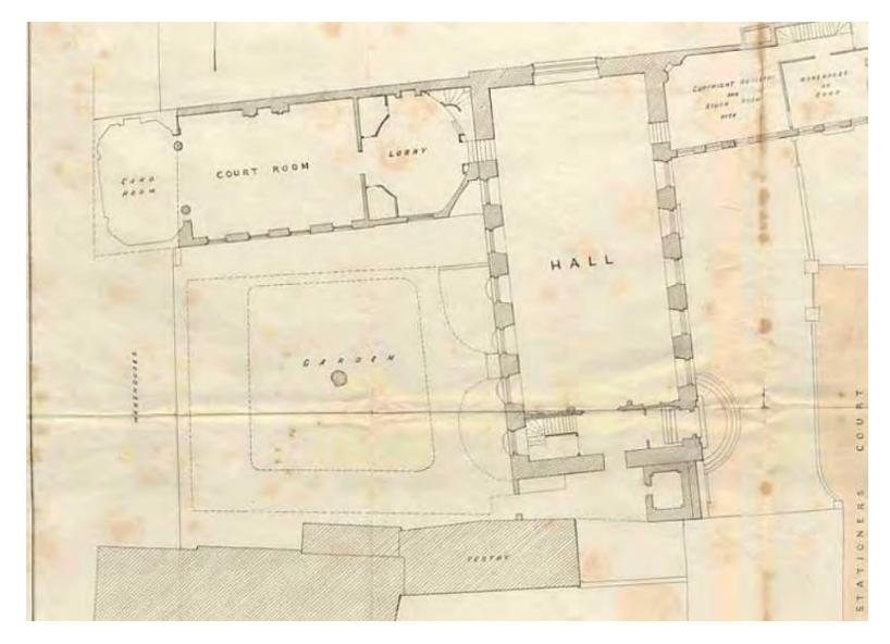
Figure 27: c.1870 Plans showing the layout of the Hall complex and Gardens. Note the layout appears to indicate a door to Hall undercroft which is no longer existing (TSC/1/G/06/04/01/51).
