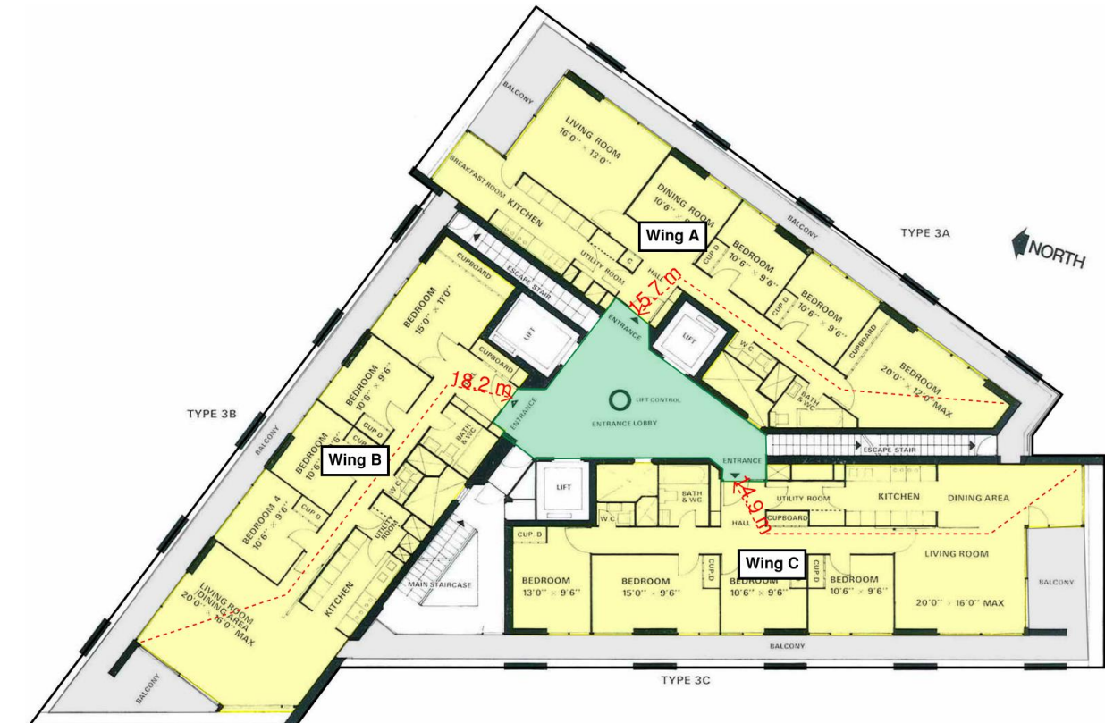
Figure 11: Extended travel distance for single means of escape for PRMs
