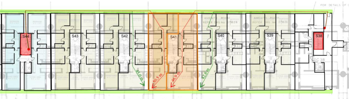
Figure 23: Hose coverage shortfall area shown in orange
