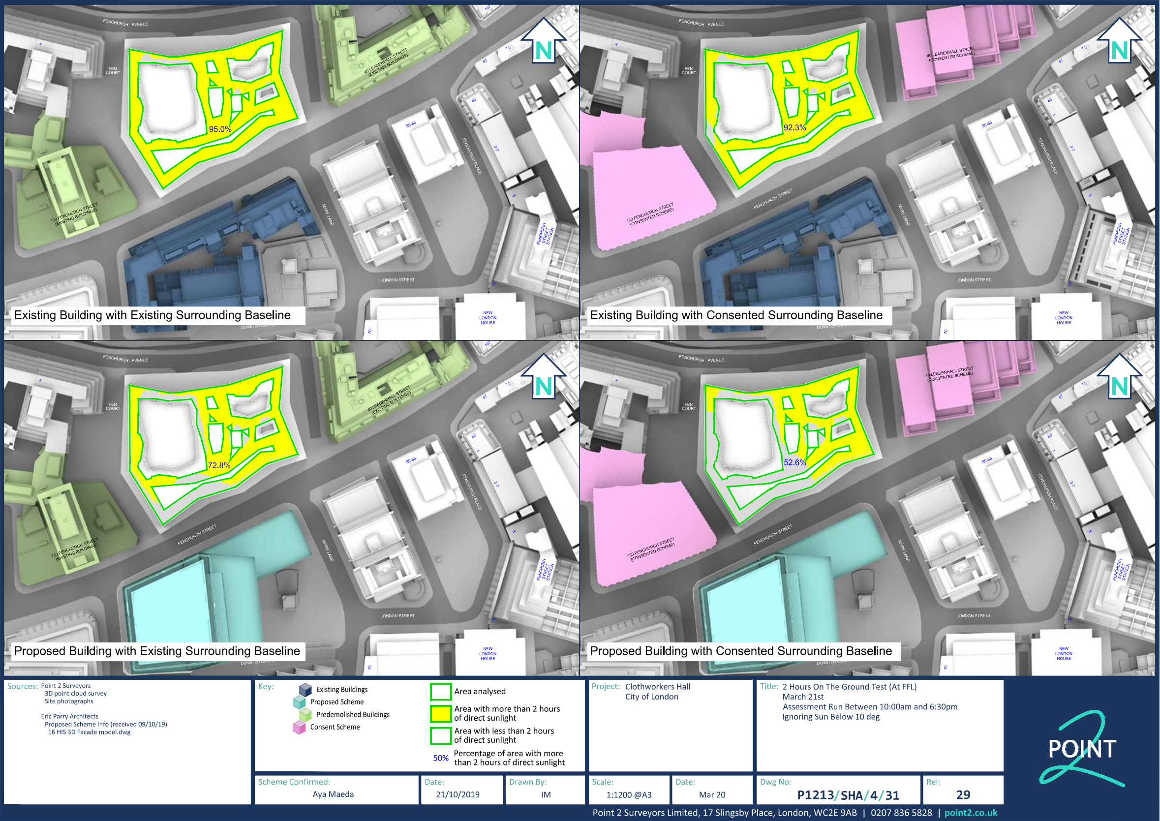
Figure 03: Point 2s Overshadowing Assessment
