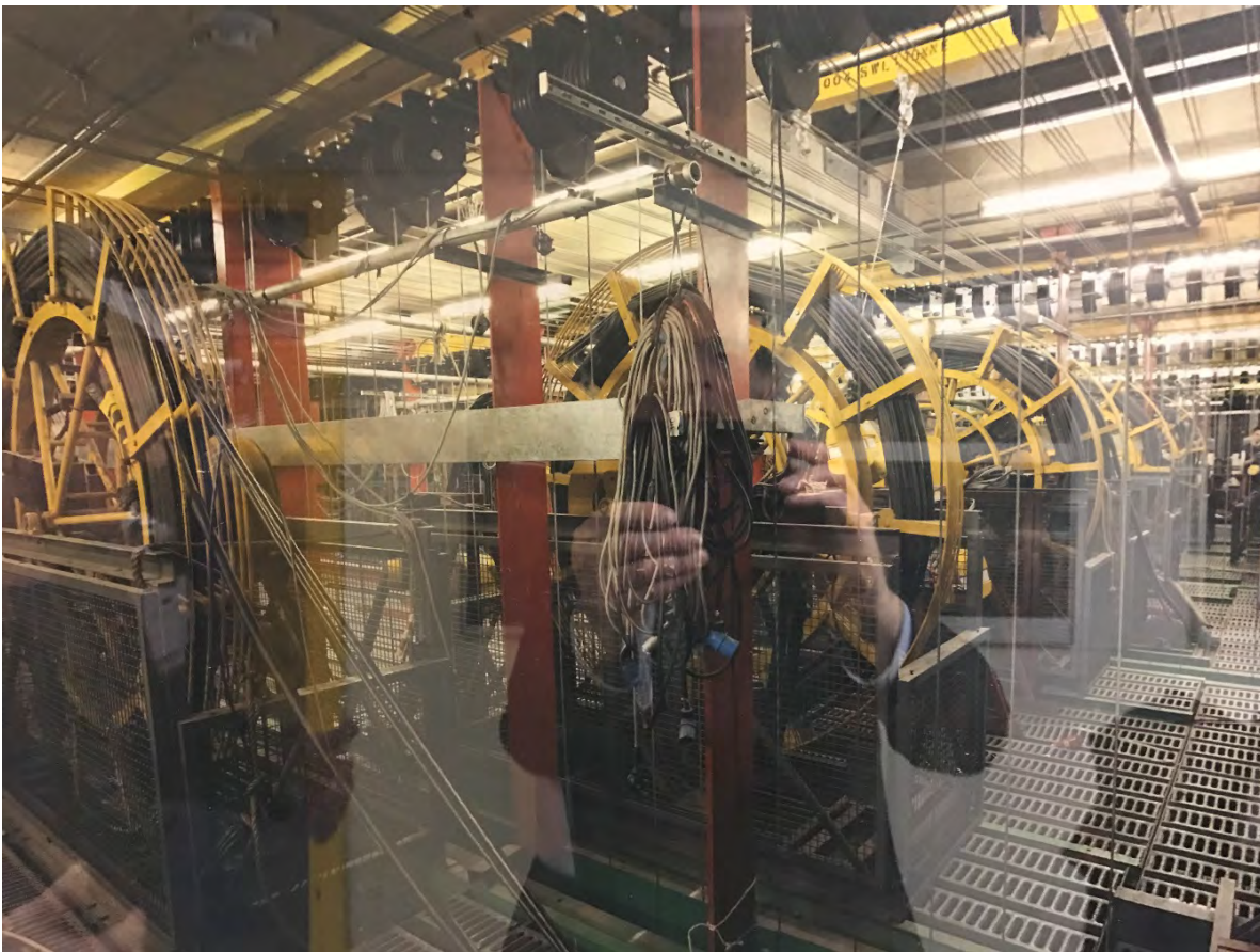
Record photographs of original scene flying machinery (now stored in Car Park 5, Cage 22)
