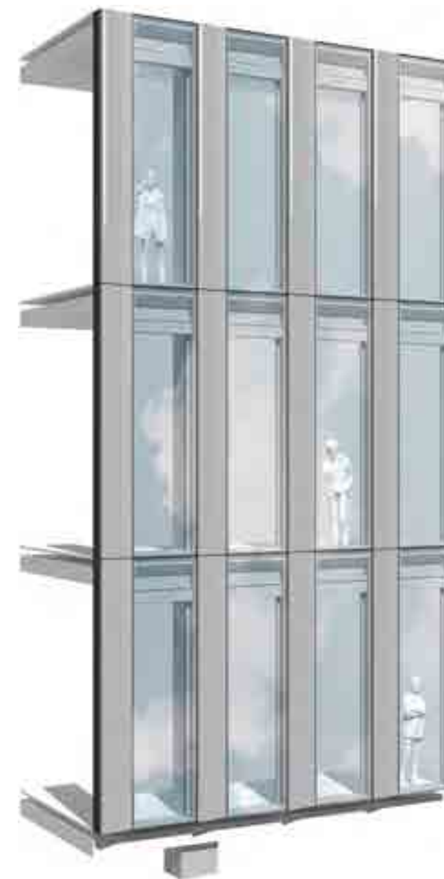
3 East block side façade 53% solid to glass ratio
