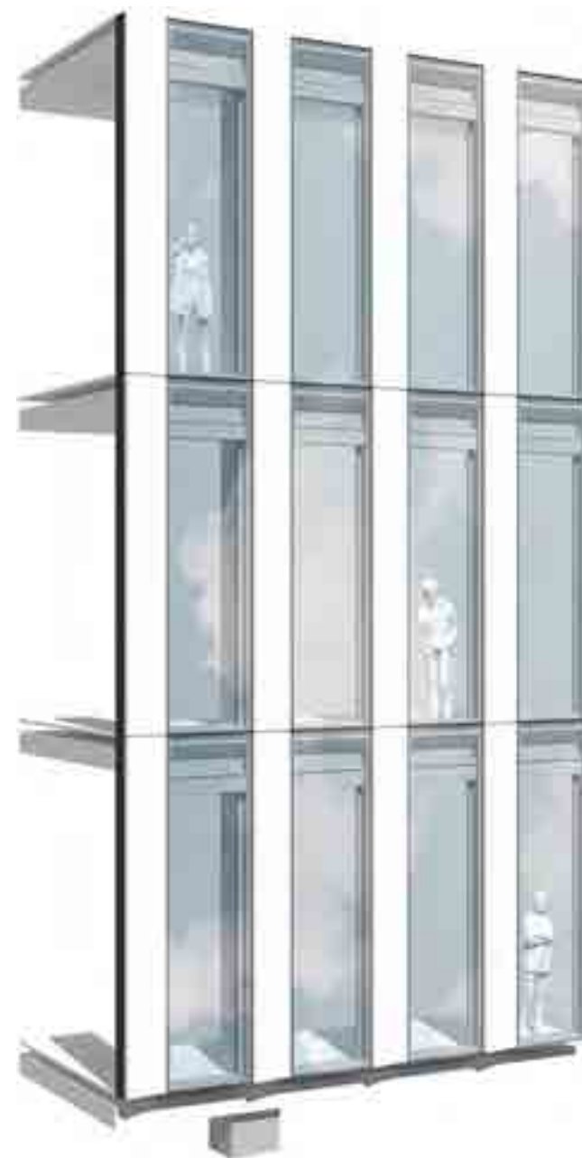
1 West block side façade 53% solid to glass ratio
