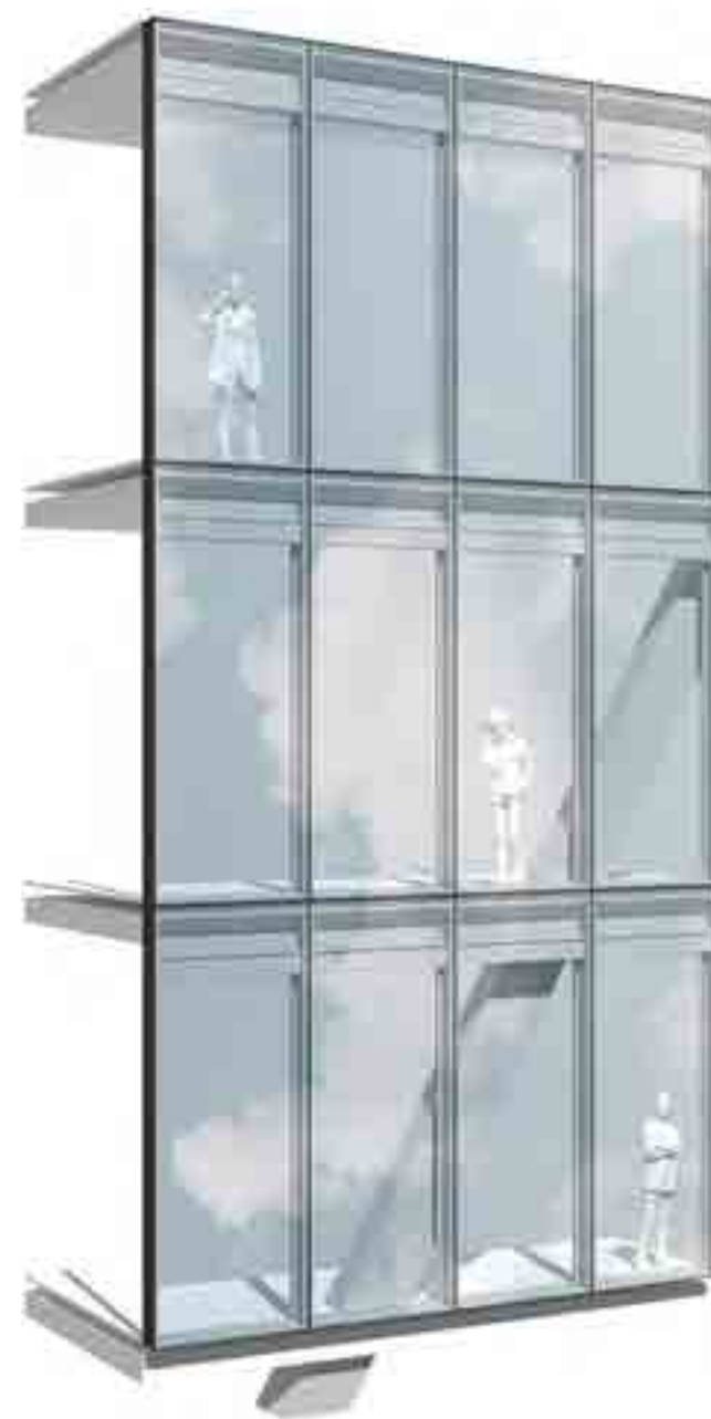
2 End bay façade 27% solid to glass ratio
