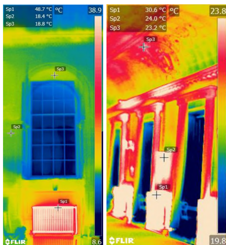
Figures 48 & 49. IRT images showing the warmed buoyant air rising from the convective radiators to heat the ceiling above.
