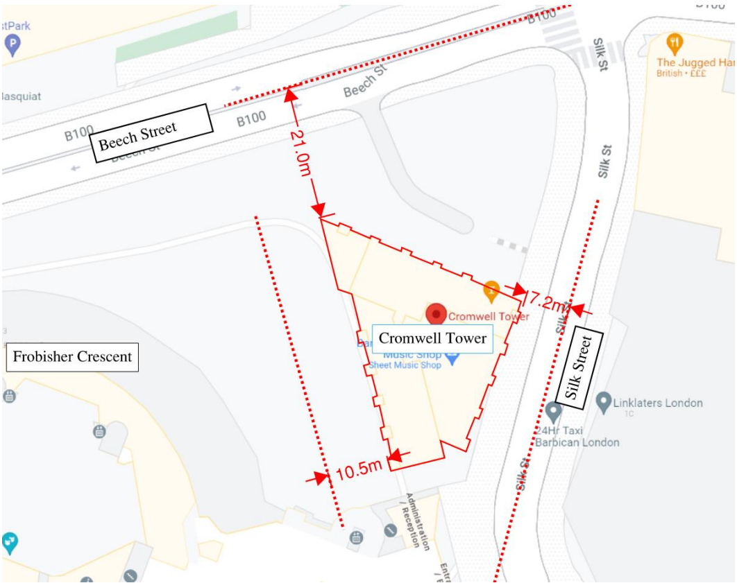
Figure 19: Existing arrangement for Cromwell Tower and adjacent buildings
