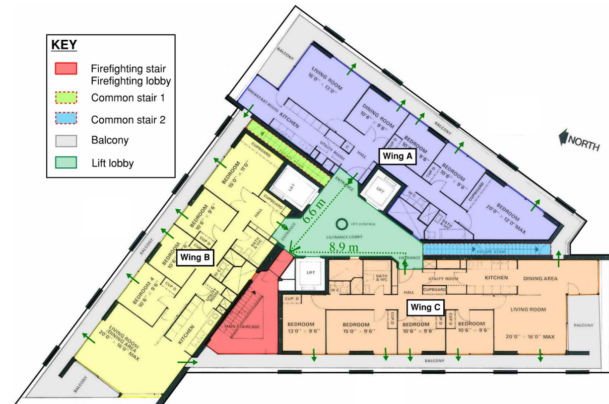
Figure 6: Travel distance in the unvented lift lobby to the firefighting stair
