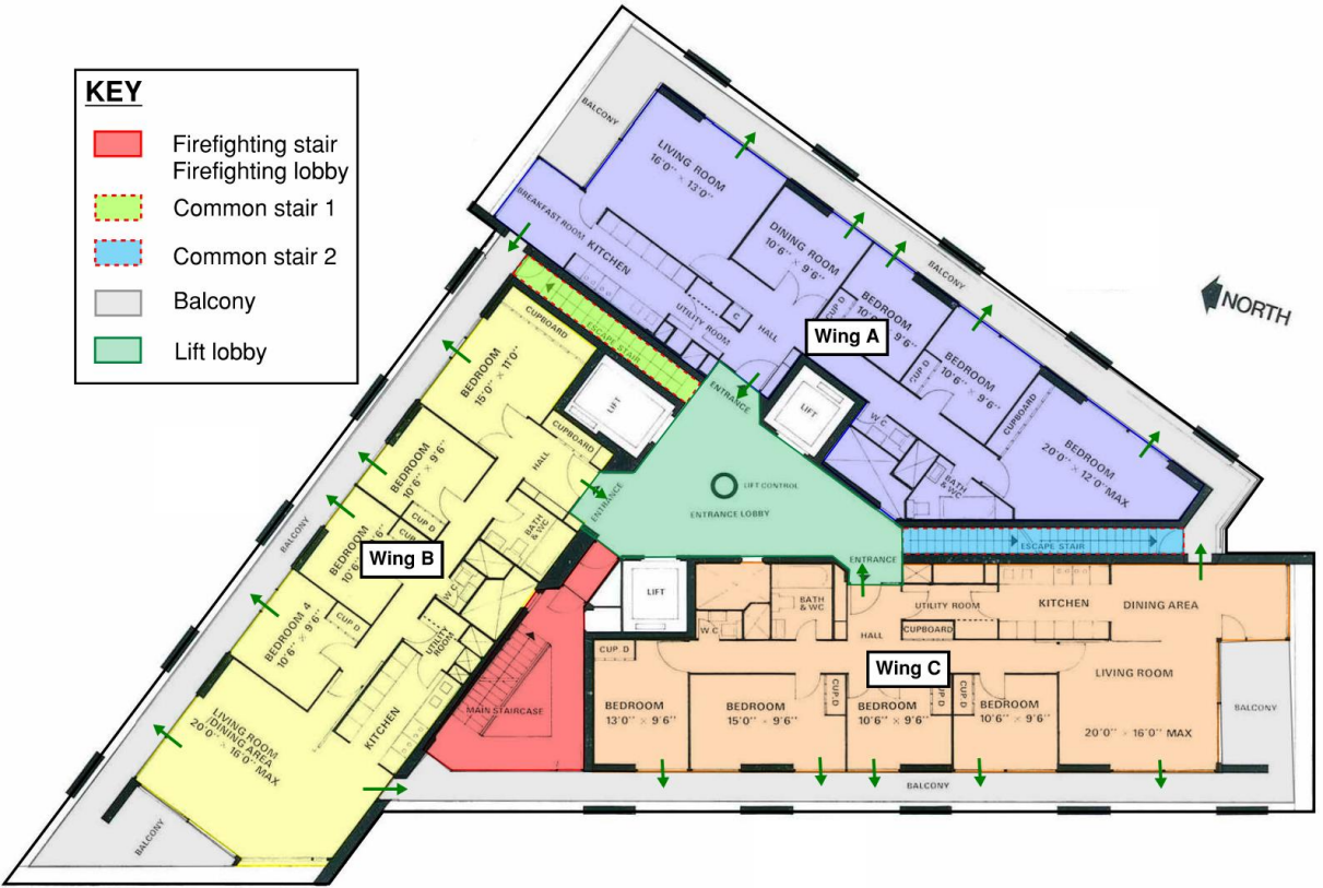
Figure 5: Available egress routes for a typical flat layout
