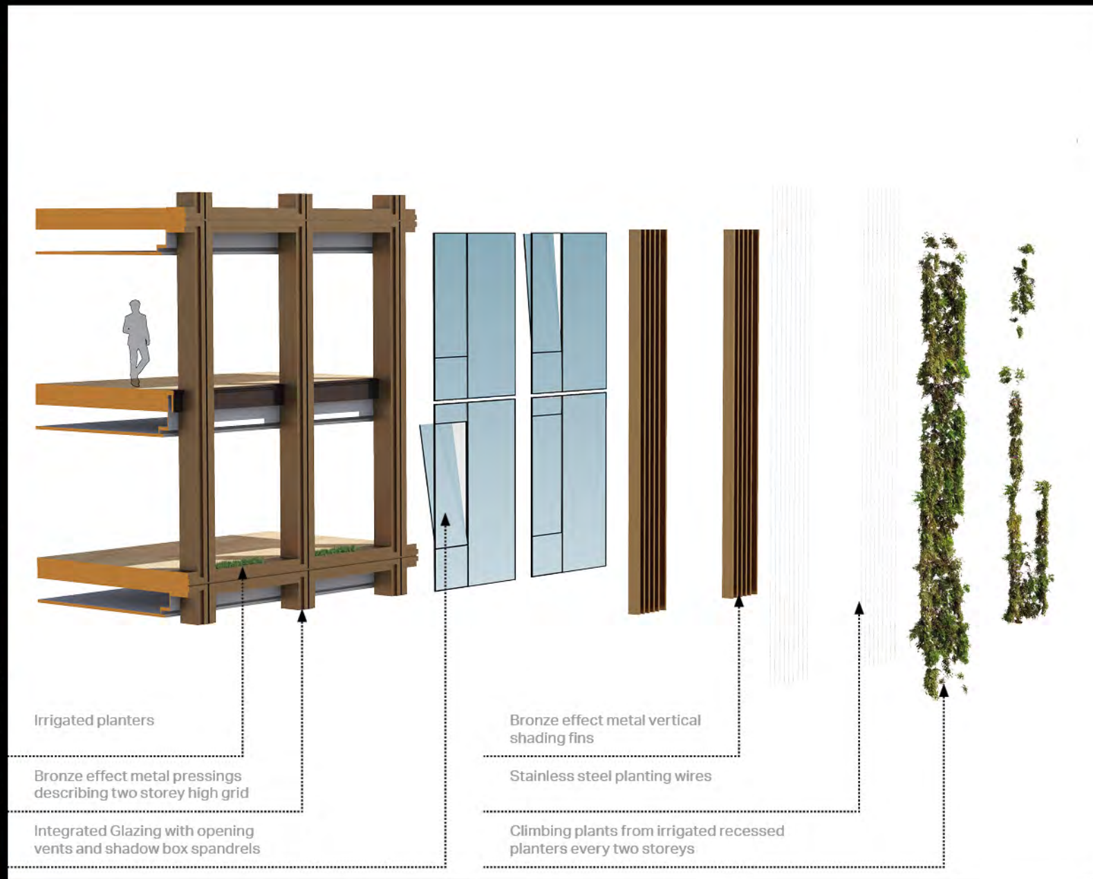
Urban Greening - Facade
