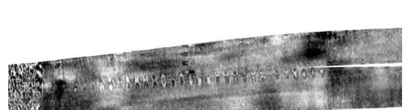
Figure 6: Possible Tie/Dowel bars at 0.20m deep.
