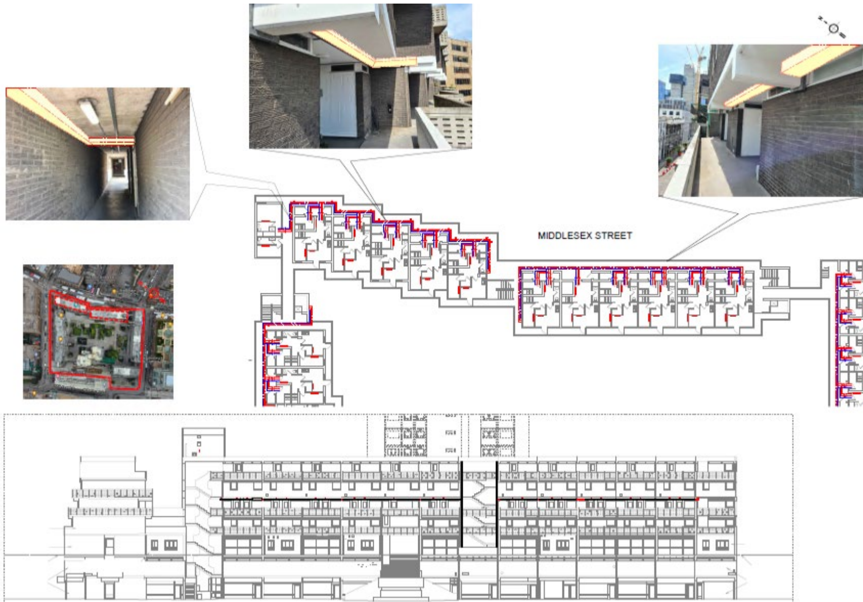
Middlesex Street external facing 4 th floor proposed heating distribution system
