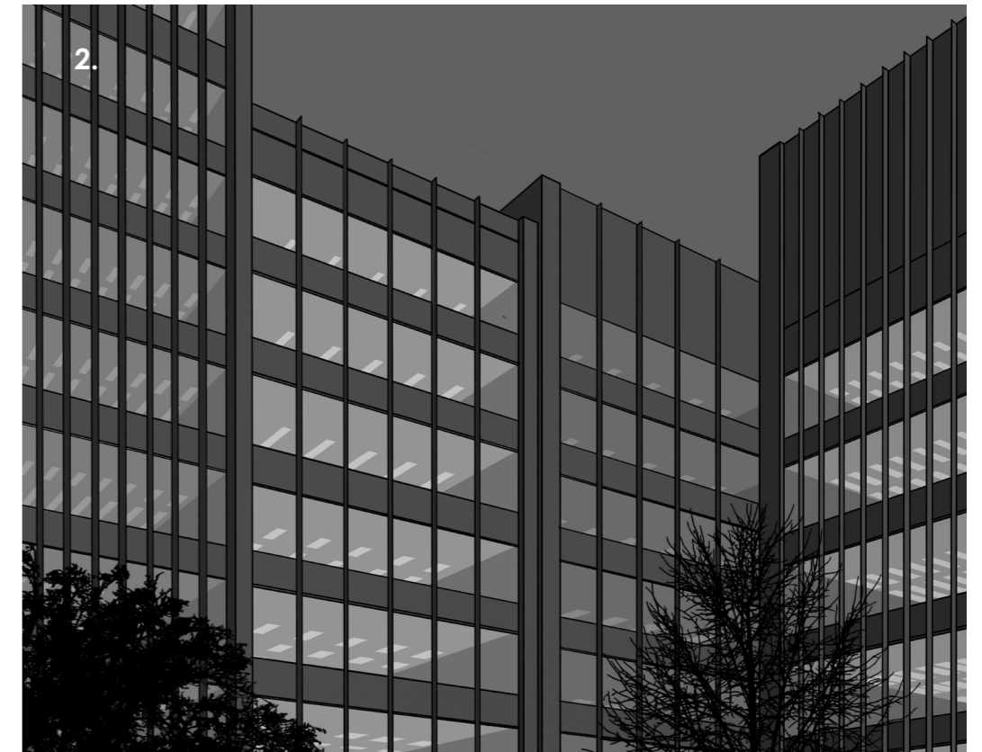
2. Blinds, coatings, frit patterns and other façade design techniques can help reduce the visibility of interior lighting at night while occupants can still perform their tasks. All developments should switch off the internal lighting when the building is not occupied.
