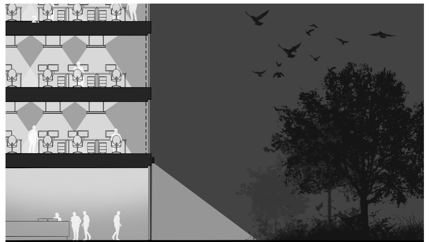
2. Strategically located internal illumination, carefully detailed glazing facades and good optical control on for external lighting can help prevent light trespass intrusion into green areas spaces and birdstrike.
