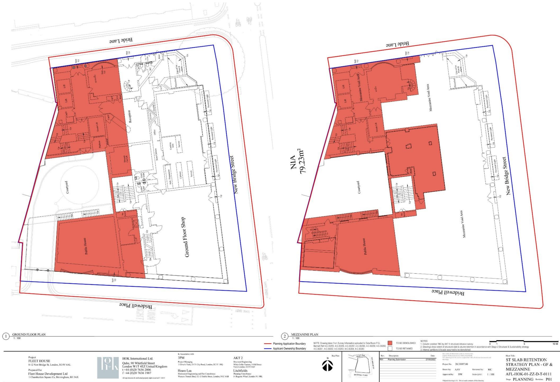
Proposed Building Plans : Ground & Mezz Retention Strategy
