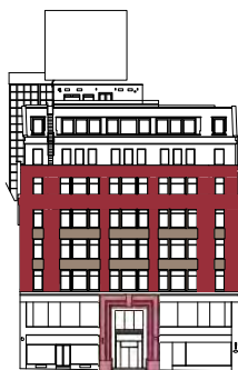
Diagram of existing elevation with retained portions highlighted
