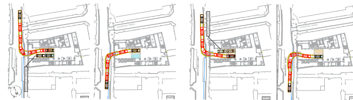
Vehicle entry and egress tracking (North lift)
