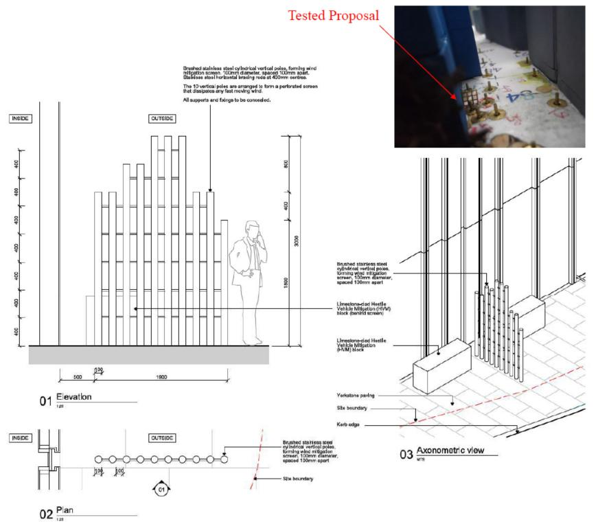
A screen of 2m x 2m (50% solid) was wind tunnel tested and presented in the planning application.
