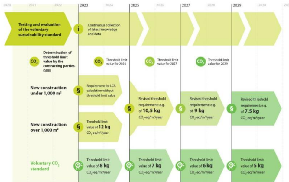
Figure 18: Step-by-step phasing and scaling up of CO 2 requirements within the National Strategy for Sustainable Construction, Source: Buro Happold and Danish Ministry of the Interior and Housing (2021).
