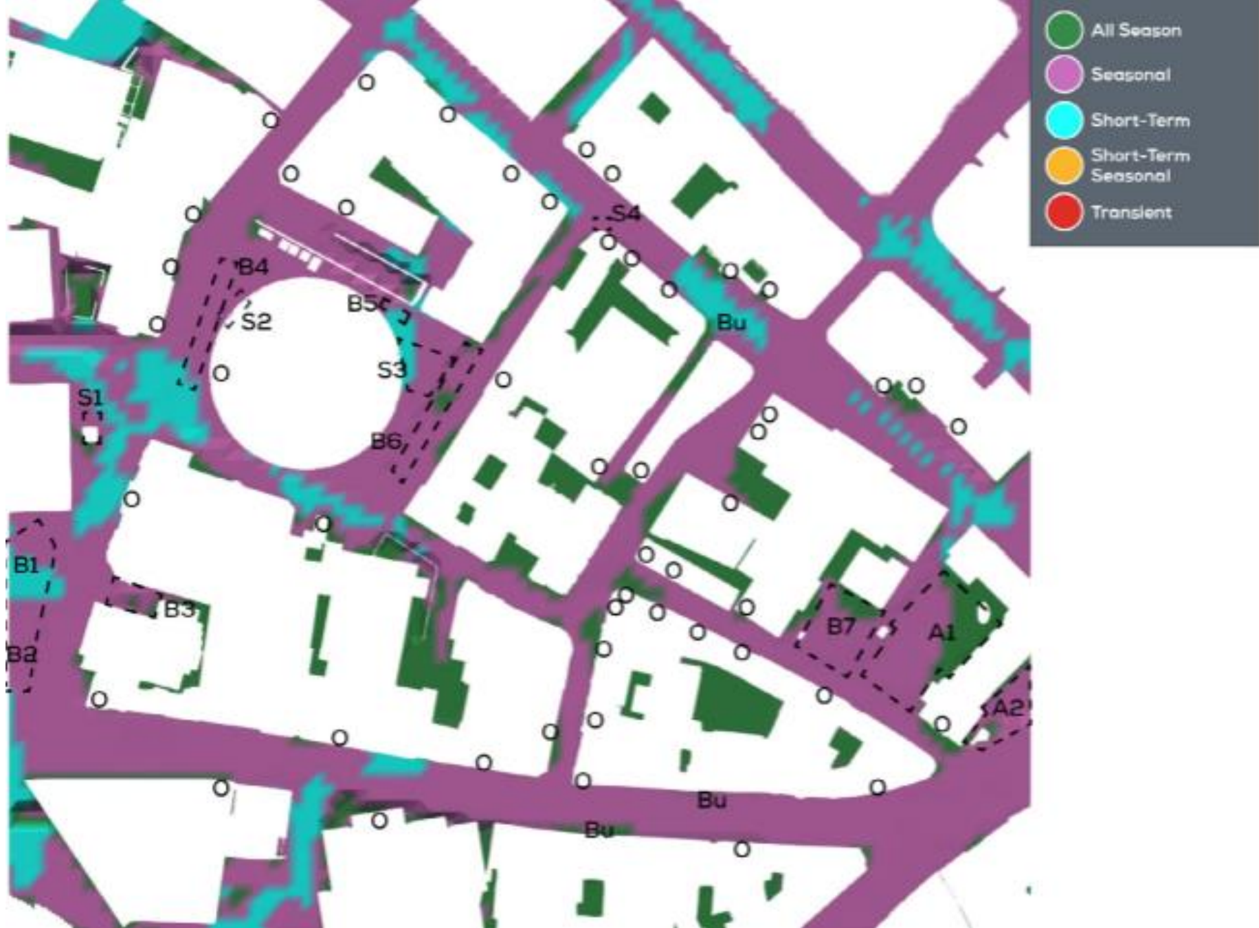
Thermal Comfort at Ground Level, Configuration 1 (Existing Building with Existing Surrounds)
