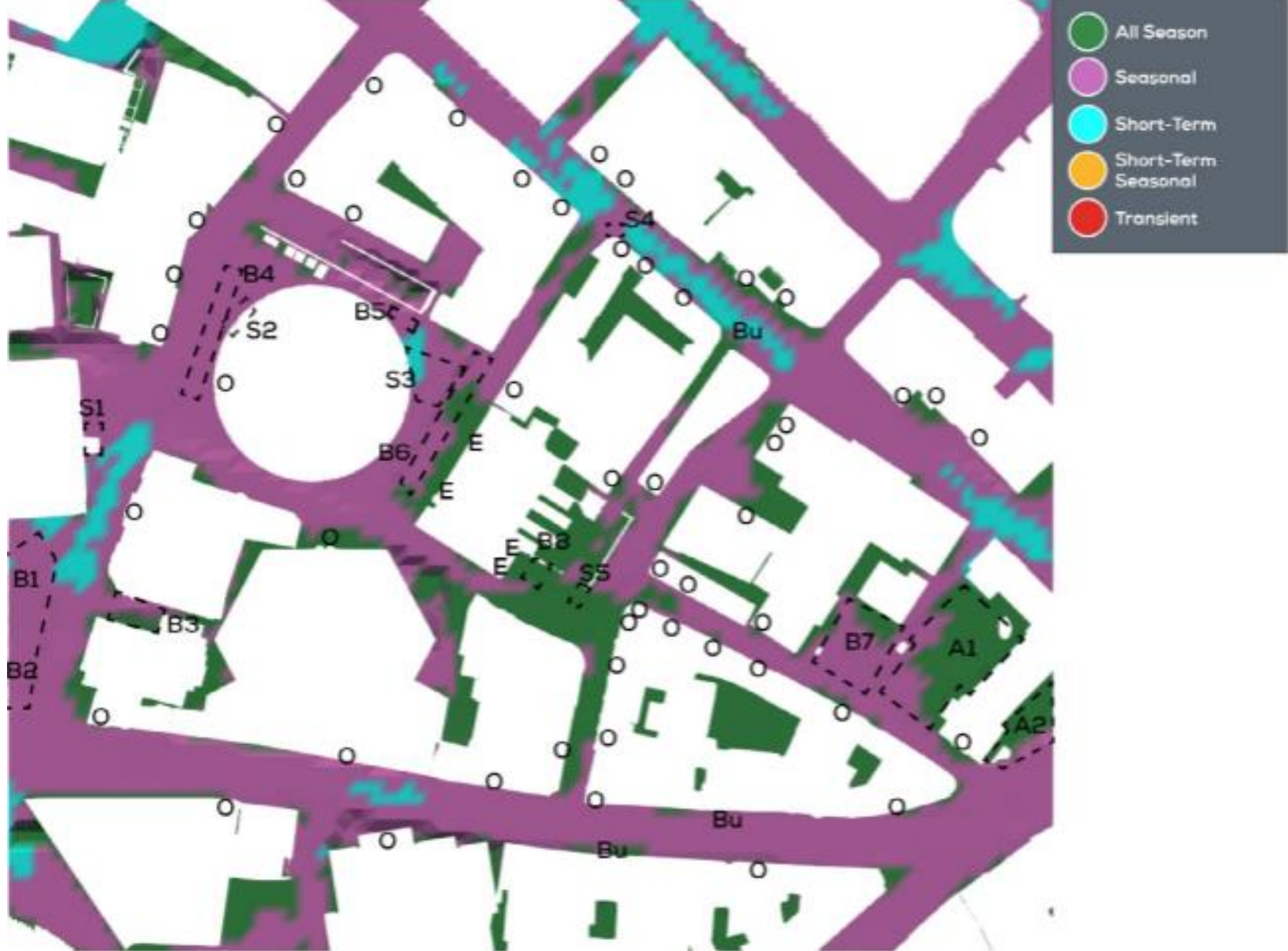
Thermal Comfort at Ground Level, Configuration 3 (Proposed Development with Tier 1 Cumulative Surrounds)
