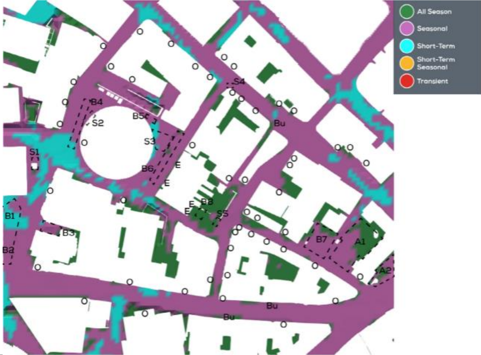
Thermal Comfort at Ground Level, Configuration 2 (Proposed Development with Existing Surrounds)
