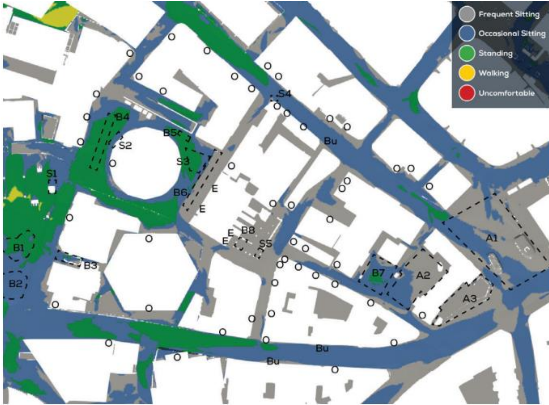
Windiest Season Conditions at Ground Level, Configuration 4 (Proposed Development with Tier 1 Cumulative Surrounds)
