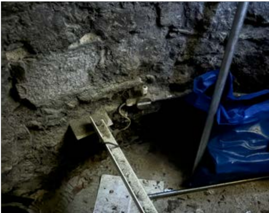
Fig. 83 Steel angle to support the verticality testing equipment
