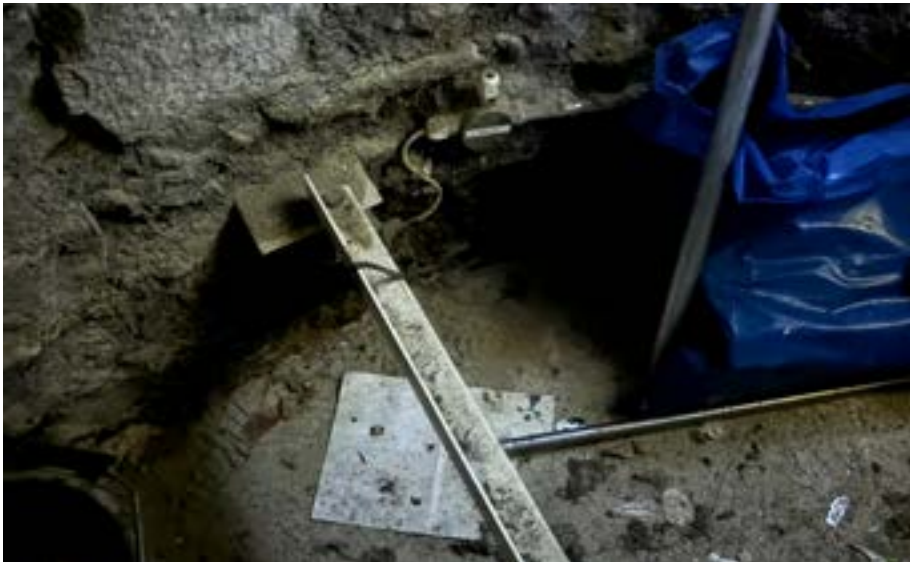
Fig. 7 Photo of steel angle locating survey plumb base point, 2024
