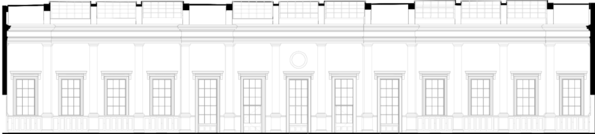
Image 2: Proposed Internal Elevation of South Facing Windows in the Long Room with Lowered Central Bay
