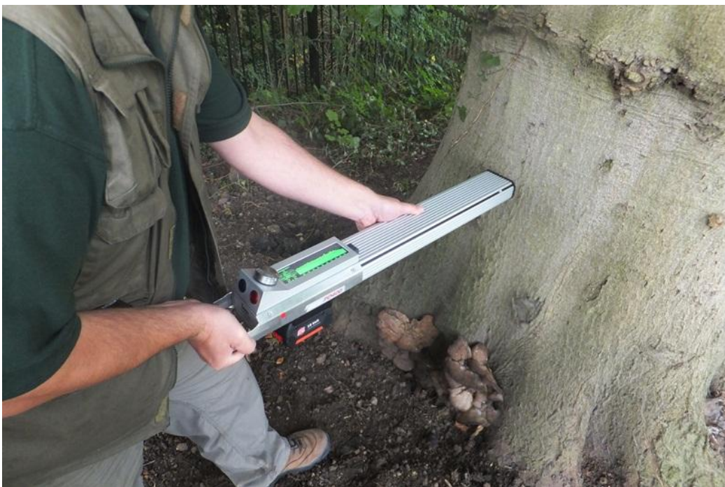
Figure 2: Resistograph being used to test for internal decay
