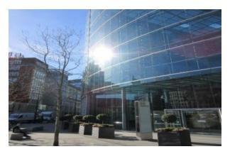
When the sun reaches the building at a glancing angle, more of it is reflected. For clear double glazing, the reflectance rises to 15% if the sun is at 45 degrees to the glazing, 22% at 60 degrees, and 49% at 75 degrees. Glare also depends on the angle of the sun and the angle at which the building is viewed.
